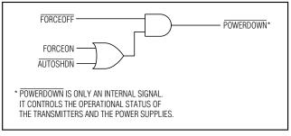
Figure 3d. Power-Down Logic
