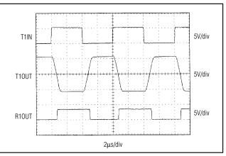
Figure 11. MAX3224E/MAX3226E/MAX3244E Loopback Test Result at 250kbps
