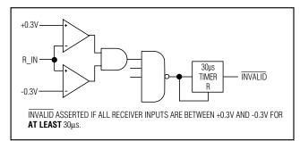
Figure 3a. INVALID Functional Diagram, INVALID Low
