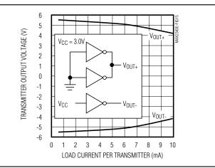
Figure 13b. MAX324\_E Transmitter Output Voltage vs. Load Current per Transmitter
