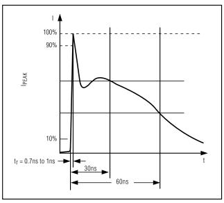
Figure 7b. IEC1000-4-2 ESD Generator Current Waveform
