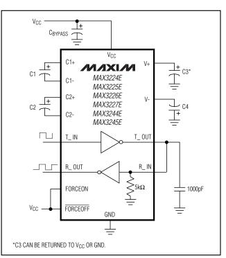
Figure 9. Loopback Test Circuit
