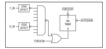
Figure 3c. AutoShutdown Plus Logic
