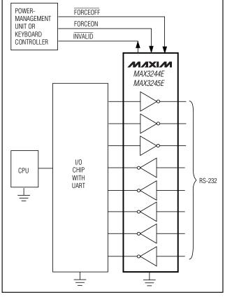
Figure 1. Interface Under Control of PMU
