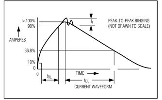
Figure 6b. Human Body Current Waveform
