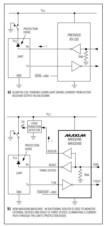
Figure 2. The MAX3244E/MAX3245E detect RS-232 activity when the UART and interface are shut down.
