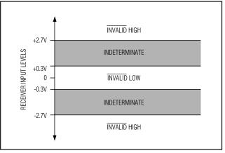
Figure 4a. Receiver Positive/Negative Thresholds for INVALID
