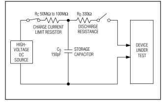
Figure 7a. IEC1000-4-2 ESD Test Model
