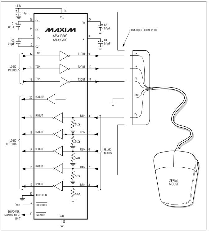
Figure 13a. Mouse Driver Test Circuit
