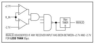
Figure 3b. INVALID Functional Diagram, INVALID High
